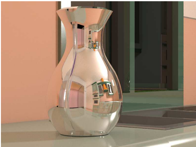
Figure 5: Vase made of perfect specular material with obscurances computed as in figure 7b. It's a 800 \times 600 px image and it takes 2108 seconds to compute.
